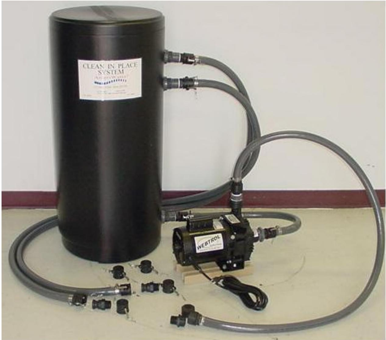
1. Remove the hoses and pump from the CIP tank (pump, hoses and fittings are shipped inside the tank from the manufacturer).
